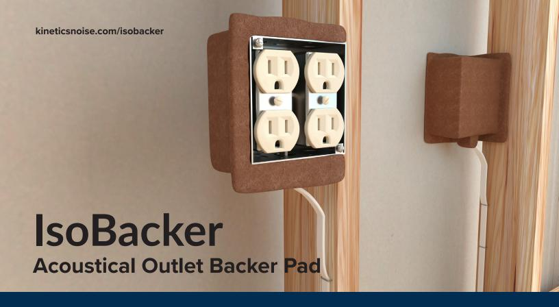
Unsealed outlet boxes are known sound leaks in stud wall assemblies. A wall designed for noise control will not perform to expectations when outlets are unsealed, particularly when outlets are back-to-back in the same stud cavity. Kinetics IsoBacker outlet pads can be hand formed around the back of the outlet box to prevent this common sound leakage problem in stud walls.
